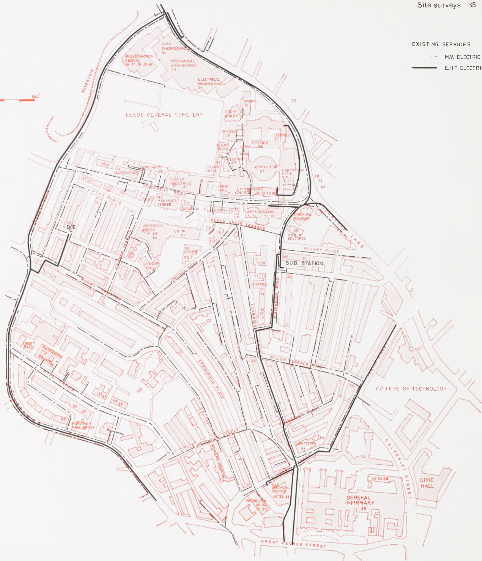
35a A survey of existing electrical mains
