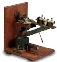
BRAGG X-RAY SPECTROMETER ENGLAND, 1910-1926
